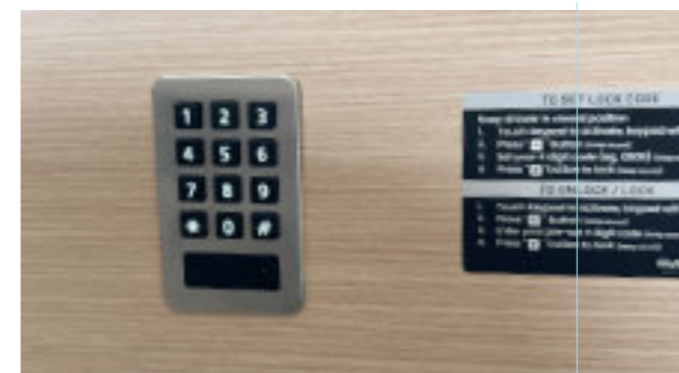
electronic keyless lock with backlit (optional)
